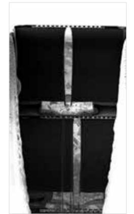
Figure 15: Three layers stacking has been demonstrated in FAB2ASM project: 50µm thin dies bonded on substrate forming a 3 layer-stack.
