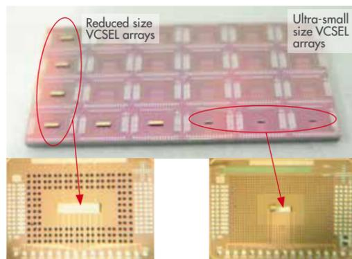
Figure 14: The picture of the Si-bench with reduced and ultra-small size VCSEL arrays assembled using liquid assisted self-alignment (SA) process. Simultaneous SA process of multiple arrays was demonstrated
