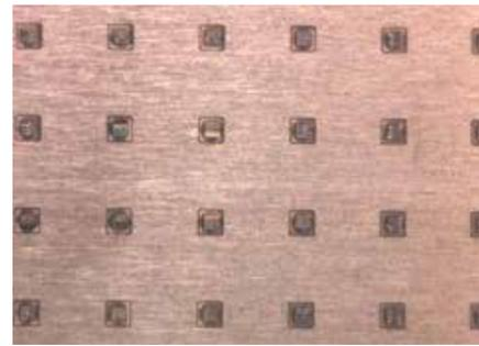
Figure 12: Results of hybrid microassembly of dies on lead frame with NXP high-speed die bonding machine. The assembled dies has a good position accuracy of about 2µm on the substrate. Higher accuracy can be reached with better defined patterns.
