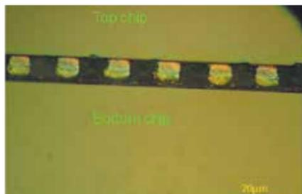
Figure 7: Optical photograph showing cross-section, 7.5 μm diameter, 20 μm Cu/Sn bumps, assembled using capillary self alignment [7]
