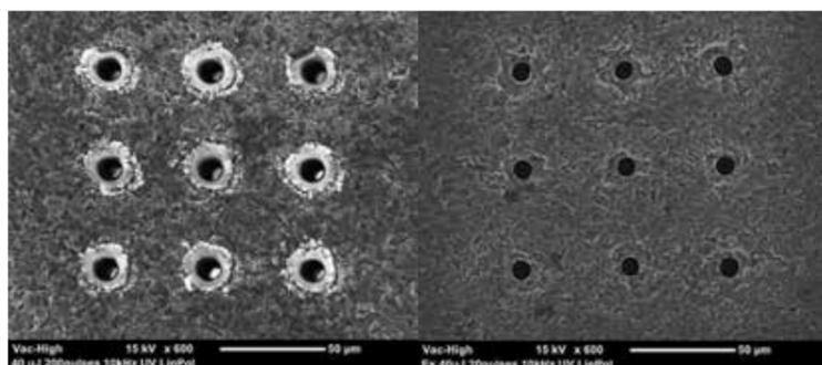
Figure 8. SEM images of the entrance and exit sides of holes drilled using 343nm (ultraviolet) laser light with 40 μJ pulse energy and repetition frequency of 10 kHz in 200 μm thick Si wafer
