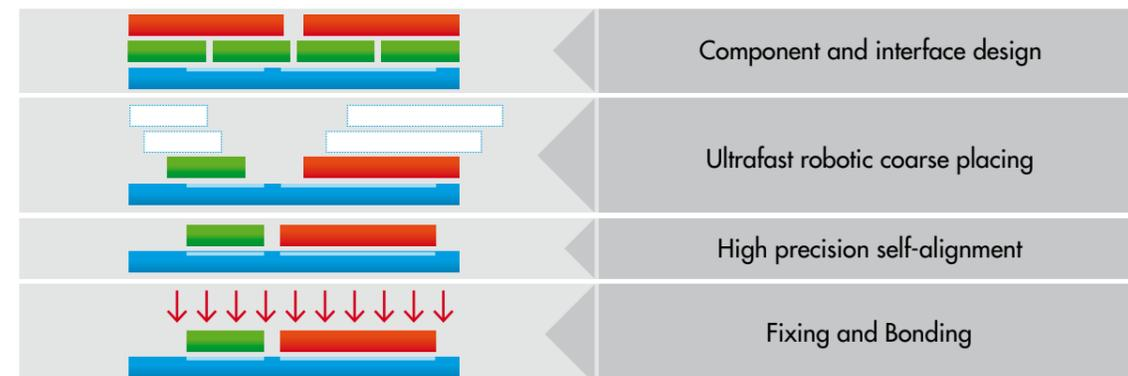
Figure 1: Main process steps of hybrid microassembly
