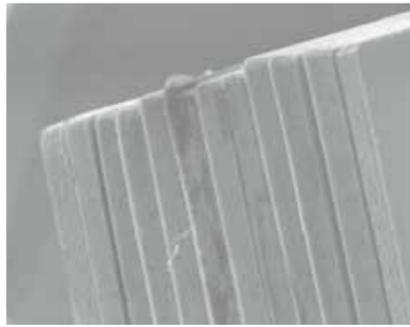
Figure 5: Hybrid microassembly of 12 layers of 1 mm x 1 mm die with thickness of 10 μm [4].
