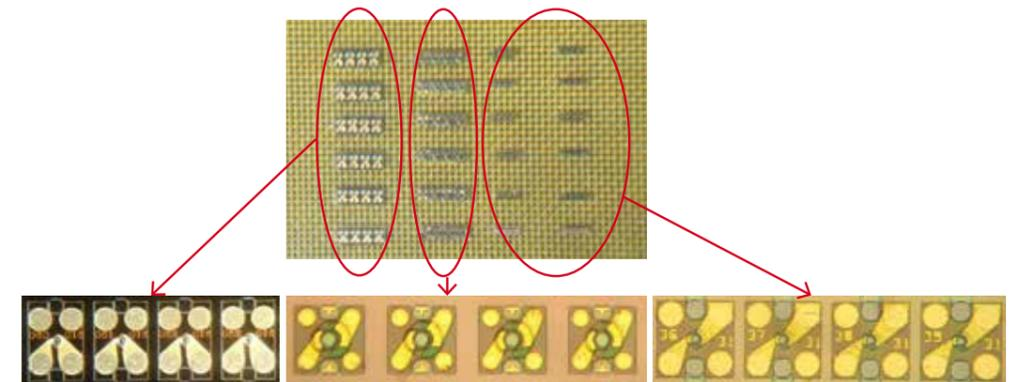
Figure 2: Fabricated 1490 nm VCSELs with different footprints
