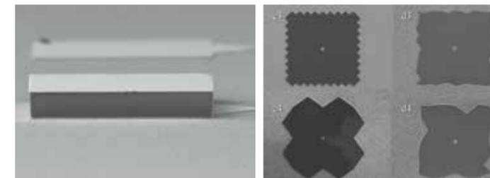
Figure 3: surface design. Left: self-aligned chips; Right: low precision patterns.
