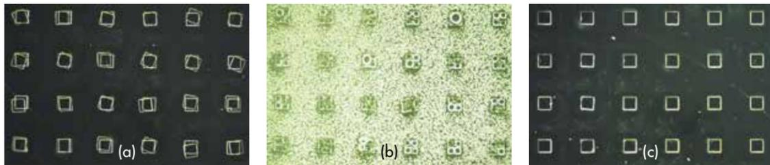
Figure 6: Parallel hybrid microassembly of 30 microchips with water mist: a) 200 μm x 200 μm x 30 μm chips are placed on the top of a matrix of 30 receptors of the same size with random placement error; b) water droplets are delivered in the form of the water mist; c) the placement errors are corrected and all the chips are aligned with the receptors
