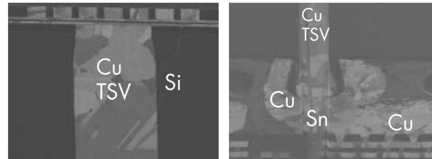
Figure 11: Focused ion beam cross-sectional SEM images of TSV connecting to the metal wiring on the top of the chip (left) and TSV connecting to the microbump of the bottom chip (right)
