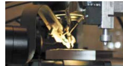
Figure 10: Hybrid micro-assembly test station ultra-thin die handling tool integrated in the front.
