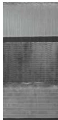
Figure 9. Multi-layer nano solders. Top: 5 nm Cu and 2 nm W; Middle: 50 nm Cu and 2 nm W; Bottom: 100 nm Cu and 2 nm W
